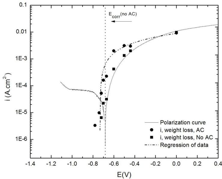
Figure 4: Effect of AC on current density of carbon steel at different DC biases.
