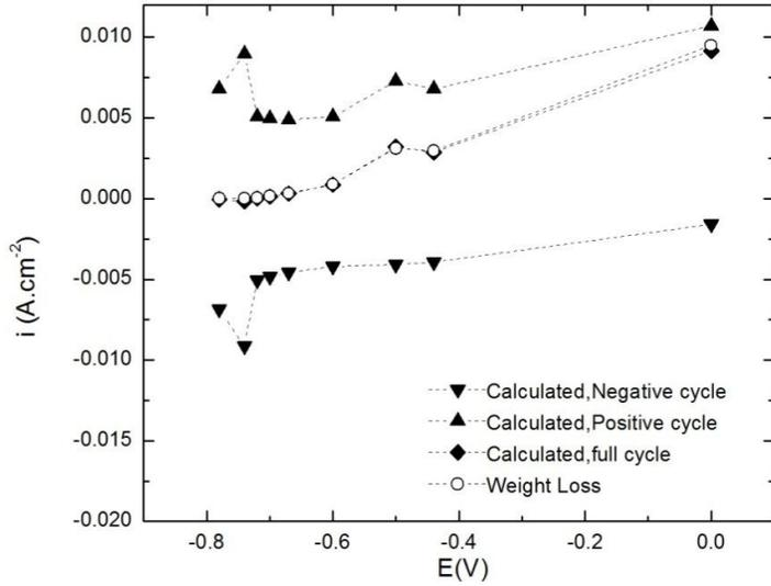
**Figure 6: Comparison of corrosion rate with AC from weight loss and three different cycles of potentiostatic test.**
