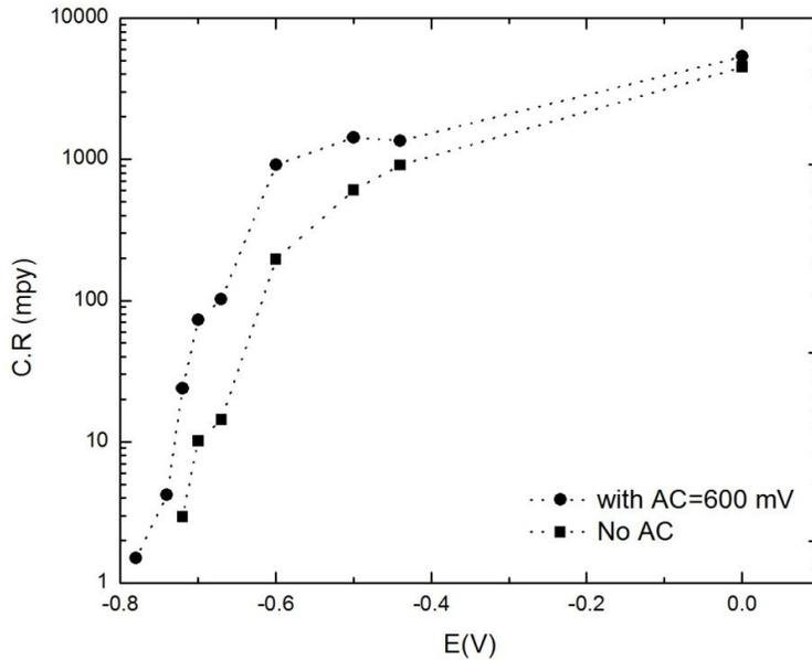
**Figure 3: Effect of AC on corrosion rate of carbon steel at different DC biases.**
