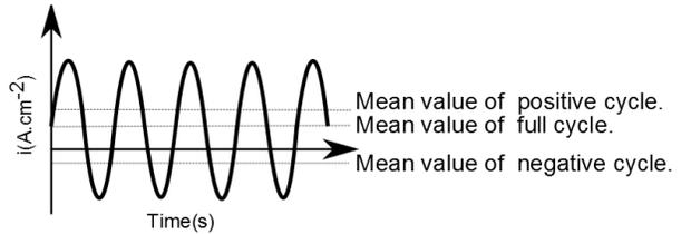
**Figure 7: Schematic of sinusoidal AC current density from potentiostatic test.**
