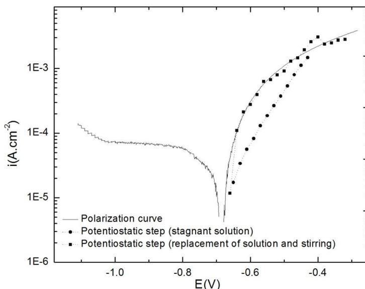
**Figure 1: Effect of solution replacement and stirring on current density.**
