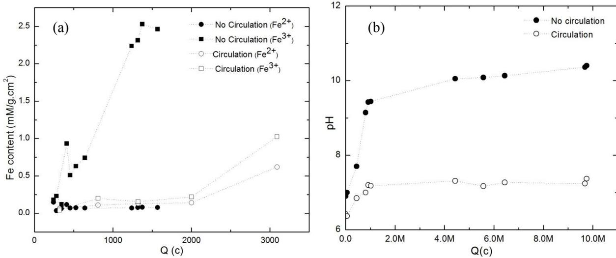
**Figure 2: Effect of solution replacement and stirring on: (a) Fe content of electrolyte at DC=-500 mV vs. SCE; (b) pH at DC=0 V vs. SCE.**
