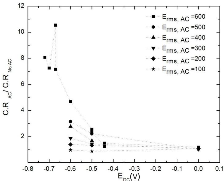
**Figure 5: Effect of different AC amplitudes on the ratio of corrosion rate with AC to the corrosion rate without AC at different DC potentials.**
